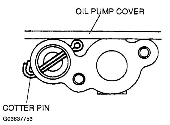
**<u>Fig. 38: Identifying Cotter Pin</u>** Courtesy of MAZDA MOTORS CORP.
