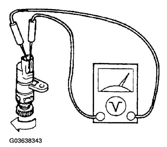
Fig. 7: Measuring Voltage Between Terminals Of Vehicle Speedometer Sensor Courtesy of MAZDA MOTORS CORP.
