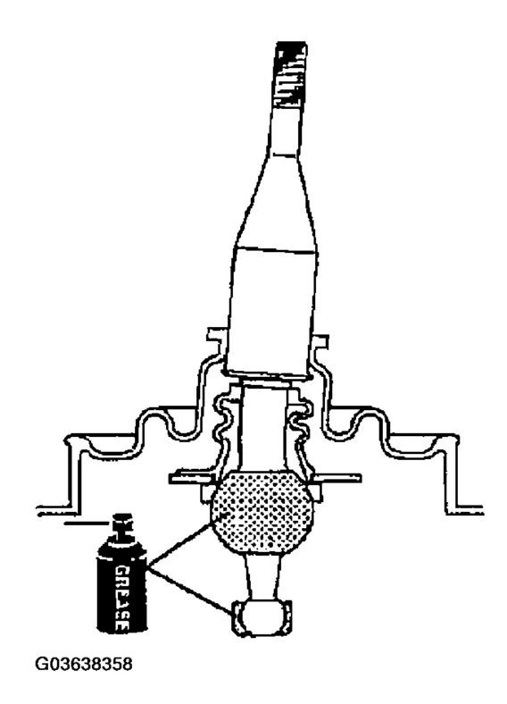
Fig. 22: Applying Grease To Shift Lever Component
