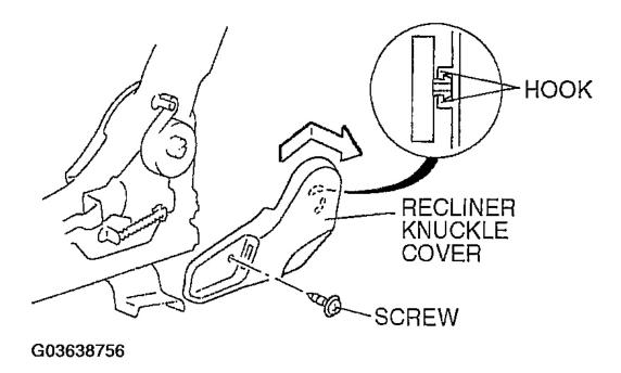
Fig. 3: Removing Reclining Knuckle Cover Courtesy of MAZDA MOTORS CORP.
