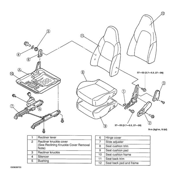
Fig. 2: Disassembling Seat - With Torque Specifications Courtesy of MAZDA MOTORS CORP.
