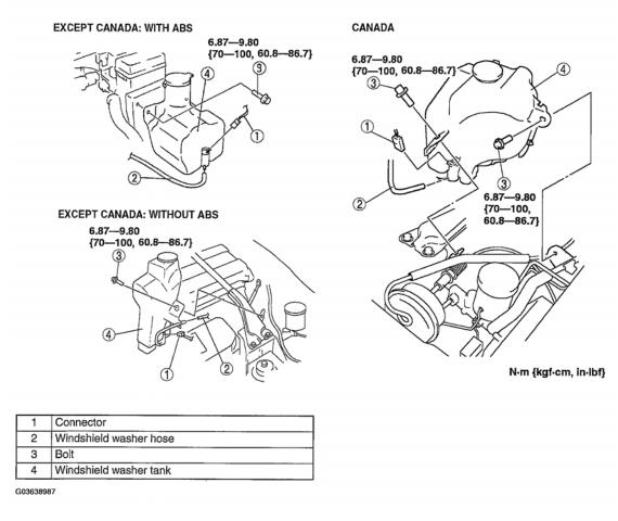
Fig. 13: Removing Windshield Washer Tank - With Torque Specifications Courtesy of MAZDA MOTORS CORP.
