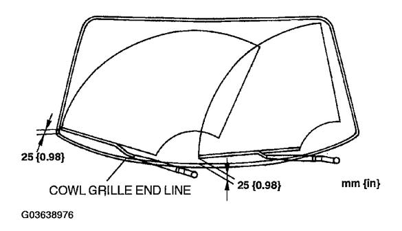
Fig. 2: Identifying Windshield Wiper Arm Height Courtesy of MAZDA MOTORS CORP.
