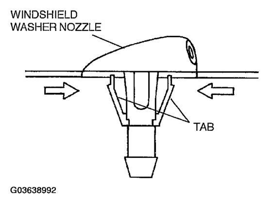
Fig. 18: Removing Windshield Washer Nozzle Courtesy of MAZDA MOTORS CORP.
