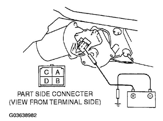
Fig. 8: Inspecting For Continuity Between Windshield Wiper Motor Terminals Using An Ohmmeter
