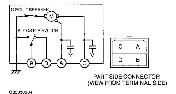
Fig. 10: Inspecting For Continuity Between Windshield Wiper Motor Connector Terminals Courtesy of MAZDA MOTORS CORP.
