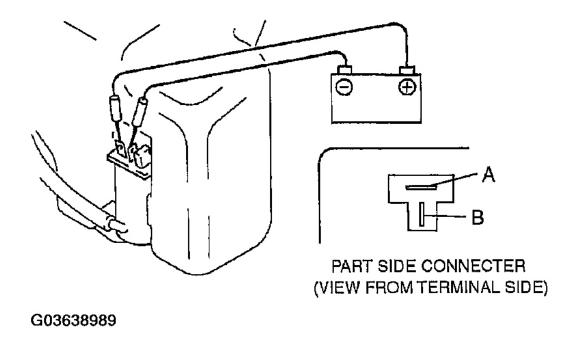
Fig. 15: Inspecting Windshield Washer Motor Courtesy of MAZDA MOTORS CORP.
