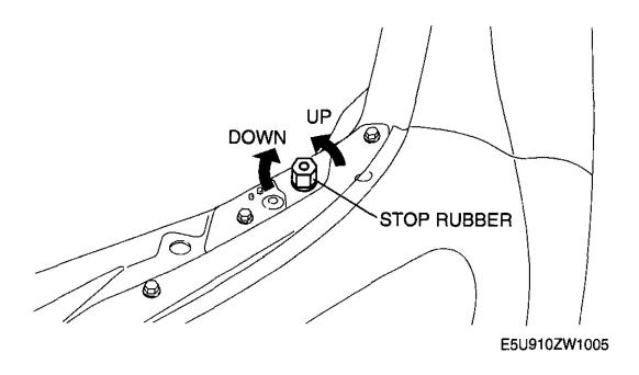
Fig. 16: Turning Stop Rubber To Adjust Height Of Hood Courtesy of MAZDA MOTORS CORP.
