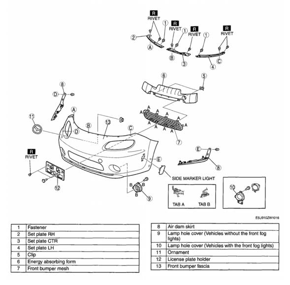
Fig. 5: Disassembling/Assembling Front Bumper Courtesy of MAZDA MOTORS CORP.
