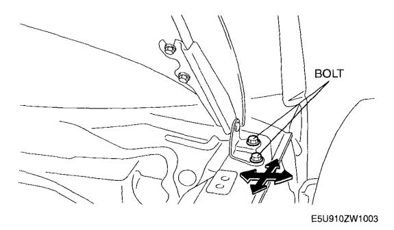
Fig. 14: Adjusting Hood Hinge Courtesy of MAZDA MOTORS CORP.
