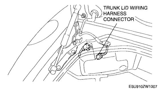
Fig. 18: Disconnecting Trunk Lid Wiring Harness Connector Courtesy of MAZDA MOTORS CORP.
