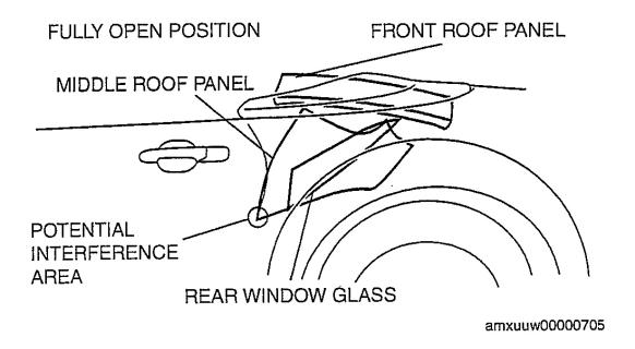
Fig. 26: Power Retractable Hardtop
