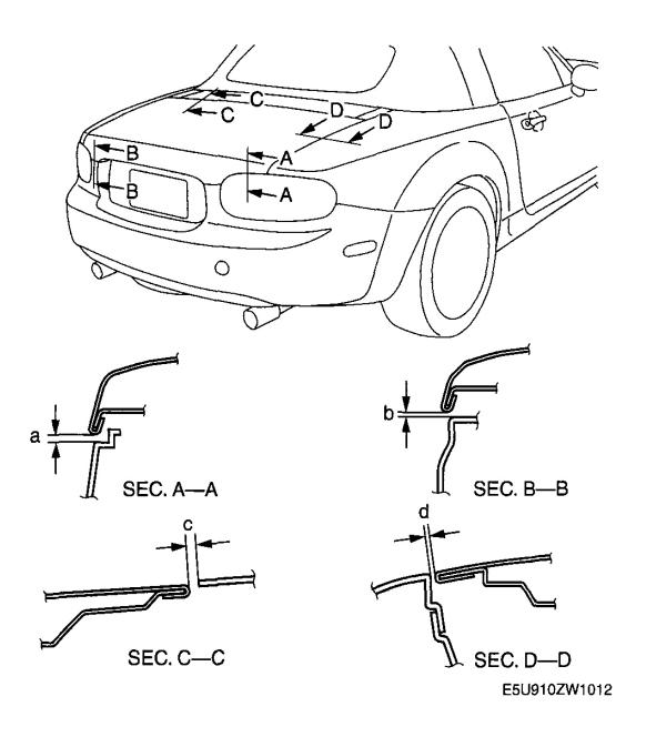
Fig. 23: Identifying Trunk Lid Standard Clearance Courtesy of MAZDA MOTORS CORP.
