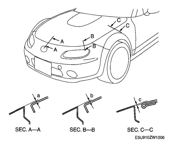
Fig. 17: Identifying Height Difference Between Hood & Body Courtesy of MAZDA MOTORS CORP.
