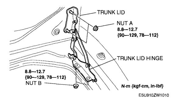
Fig. 21: Removing Trunk Lid Hinge (With Torque Specifications) Courtesy of MAZDA MOTORS CORP.
