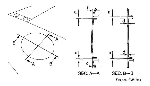
Fig. 3: Identifying Gap & Height Difference Between Fuel-Filler Lid & Body Courtesy of MAZDA MOTORS CORP.
