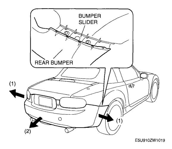
Fig. 9: Pulling Rear Bumper Ends (Wheel Arch) Outward From Bumper Slider Courtesy of MAZDA MOTORS CORP.
