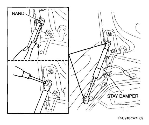
Fig. 20: Prying Out Connecting Part Of Stay Damper & Hinge With Flathead Screwdriver Courtesy of MAZDA MOTORS CORP.
