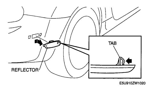
Fig. 10: Identifying Reflector Courtesy of MAZDA MOTORS CORP.
