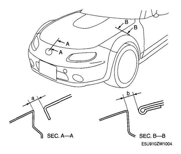
Fig. 15: Identifying Gap Between Hood & Body Courtesy of MAZDA MOTORS CORP.
