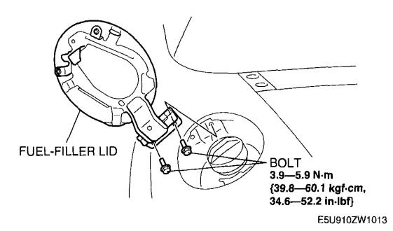
Fig. 2: Removing Fuel-Filler Lid (With Torque Specifications) Courtesy of MAZDA MOTORS CORP.
