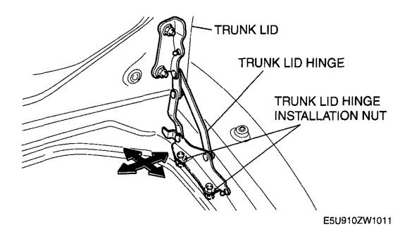
Fig. 22: Adjusting Trunk Lid Courtesy of MAZDA MOTORS CORP.
