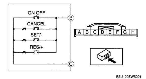
Fig. 1: Identifying Cruise Control Switch Terminals B & C Courtesy of MAZDA MOTORS CORP.
