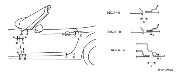
Fig. 4: Identifying Gap & Height Difference Between Door & Body
