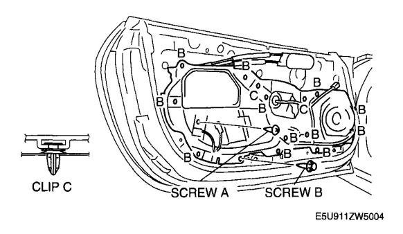
Fig. 5: Removing/Installing Door Unit Courtesy of MAZDA MOTORS CORP.
