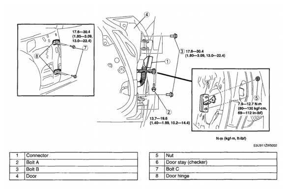
Fig. 2: Removing/Installing Door (With Torque Specifications) Courtesy of MAZDA MOTORS CORP.
