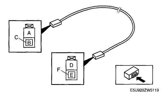
Fig. 35: Identifying AM/FM Antenna Feeder No. 2 Terminals & Connectors Courtesy of MAZDA MOTORS CORP.
