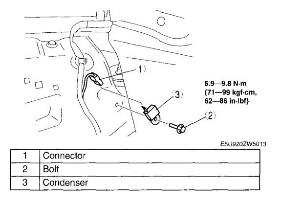
Fig. 24: Identifying Condenser (With Torque Specifications) Courtesy of MAZDA MOTORS CORP.
