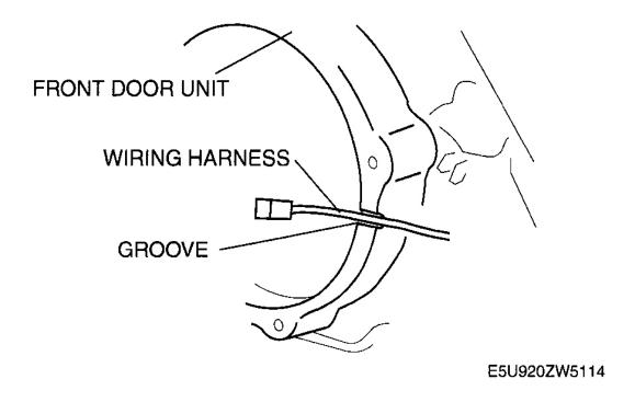
Fig. 11: Removing Speaker With Wiring Harness Passing Groove Of Front Door Module Courtesy of MAZDA MOTORS CORP.
