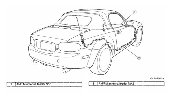
Fig. 31: Identifying Antenna Feeder Courtesy of MAZDA MOTORS CORP.
