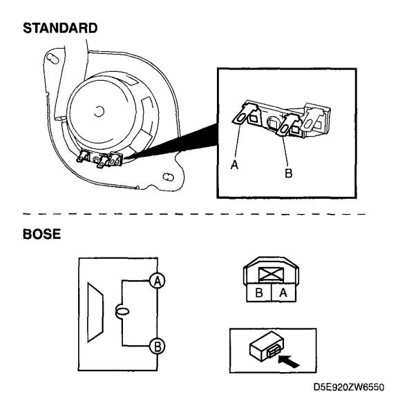
Fig. 17: Identifying Rear Speaker Terminals Courtesy of MAZDA MOTORS CORP.
