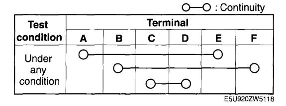
Fig. 32: AM/FM Antenna Feeder No. 1 Continuity Table Courtesy of MAZDA MOTORS CORP.
