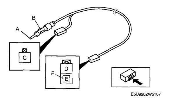
Fig. 33: Identifying AM/FM Antenna Feeder No. 1 Terminals & Connectors Courtesy of MAZDA MOTORS CORP.
