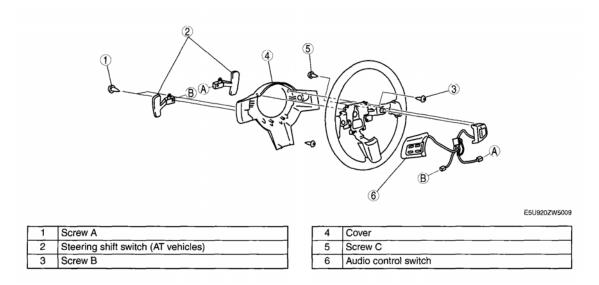
Fig. 36: Removing Driver-Side Air Bag Module Courtesy of MAZDA MOTORS CORP.
