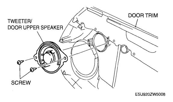
Fig. 21: Identifying Tweeter/Door Upper Speaker Courtesy of MAZDA MOTORS CORP.
