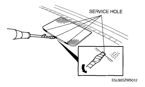
Fig. 19: Inserting Tape-Wrapped Flathead Screwdriver Into Service Hole Courtesy of MAZDA MOTORS CORP.
