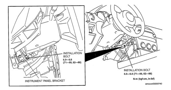
Fig. 2: Identifying Installation Bolt (With Torque Specifications) Courtesy of MAZDA MOTORS CORP.
