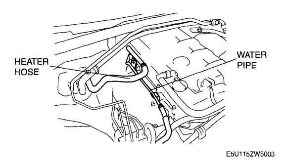
Fig. 3: Identifying Heater Hose & Water Pipe Courtesy of MAZDA MOTORS CORP.
