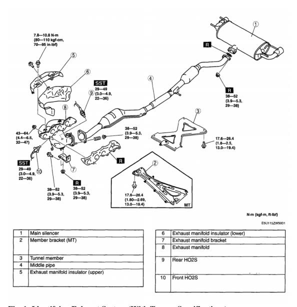
Fig. 1: Identifying Exhaust System (With Torque Specifications) Courtesy of MAZDA MOTORS CORP.
