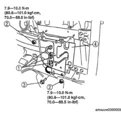
**Fig. 68: Identifying Power Retractable Hardtop Control Module Bracket Components With Torque Specifications Courtesy of MAZDA MOTORS CORP.**
