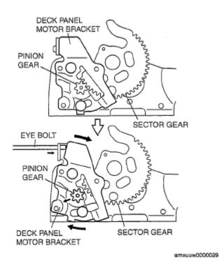
**Fig. 127: Removing Eye Bolt** Courtesy of MAZDA MOTORS CORP.
