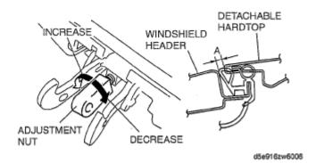
**<u>Fig. 37: Turning Adjusting Nut</u>** Courtesy of MAZDA MOTORS CORP.
