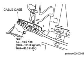
**Fig. 96: Identifying Cable Case And Nut With Torque Specifications** Courtesy of MAZDA MOTORS CORP.
