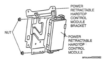
Fig. 69: Identifying Power Retractable Hardtop Control Module And Bracket Courtesy of MAZDA MOTORS CORP.
