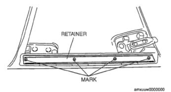
Fig. 107: Identifying Mark Around Retainer Installation Screws Courtesy of MAZDA MOTORS CORP.
