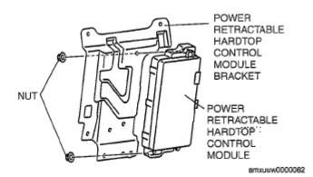
Fig. 116: Identifying Power Retractable Hardtop Control Module Bracket And Nut Courtesy of MAZDA MOTORS CORP.
