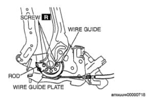
**Fig. 76: Identifying Wire Guide Plate, Wire Guide And Screw Courtesy of MAZDA MOTORS CORP.**
