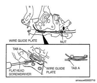
**<u>Fig. 77: Removing Tabs A</u>** Courtesy of MAZDA MOTORS CORP.
