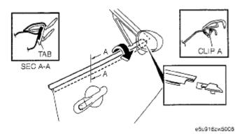
**Fig. 3: Removing/Installing Front Beltline Molding** Courtesy of MAZDA MOTORS CORP.
