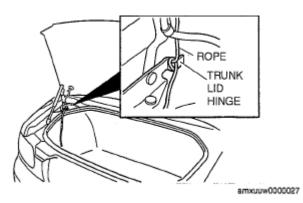
**Fig. 137: Identifying Trunk Lid Hinge** Courtesy of MAZDA MOTORS CORP.
