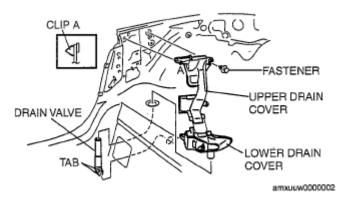
**Fig. 44: Identifying Drain Valve Components - Power Retractable Hardtop Courtesy of MAZDA MOTORS CORP.**
