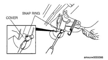
**Fig. 28: Identifying Snap Ring And Cover** Courtesy of MAZDA MOTORS CORP.
