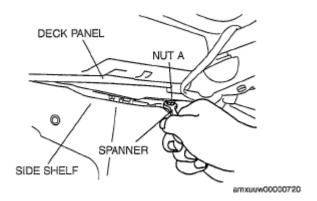
**Fig. 140: Removing Nut A** Courtesy of MAZDA MOTORS CORP.
