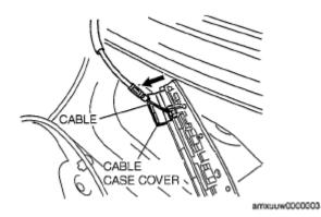
Fig. 89: Direction For Pressing Cable Courtesy of MAZDA MOTORS CORP.
