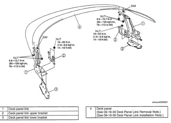
Fig. 79: Identifying Deck Panel Disassemble/Assemble Components With Torque Specifications
