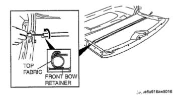
**Fig. 13: Removing Top Fabric From Front Bow Retainer** Courtesy of MAZDA MOTORS CORP.
