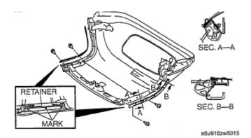
Fig. 24: Identifying Mark Around Retainer Installation Screws
