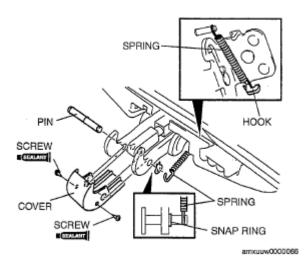
**Fig. 25: Identifying Convertible Top Adjustment Components Courtesy of MAZDA MOTORS CORP.**
