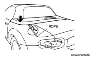
**Fig. 133: Direction Of Pulling Rope** Courtesy of MAZDA MOTORS CORP.
