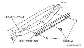
**Fig. 7: Identifying Drip Molding Components Courtesy of MAZDA MOTORS CORP.**
