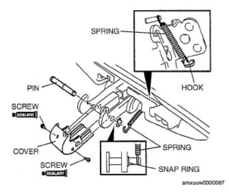
**Fig. 36: Identifying Detachable Hardtop Adjustment Components Courtesy of MAZDA MOTORS CORP.**
