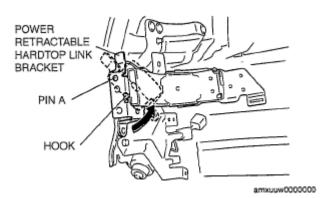
Fig. 101: Rotating Power Retractable Hardtop Link Bracket Courtesy of MAZDA MOTORS CORP.
