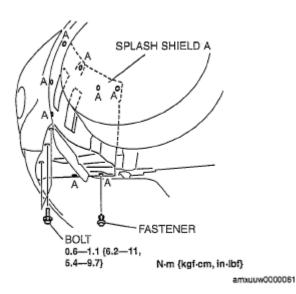
**Fig. 49: Identifying Fasteners Section With Torque Specifications Courtesy of MAZDA MOTORS CORP.**
