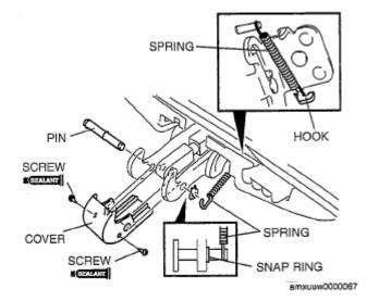
Fig. 54: Identifying Power Retractable Hardtop Adjustment Components Courtesy of MAZDA MOTORS CORP.
