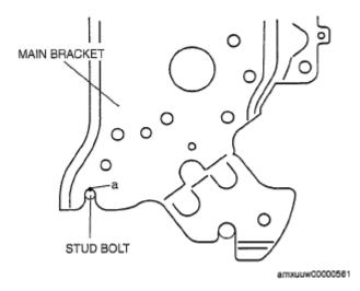
Fig. 53: Identifying Gap Between Positioning Surface Of Main Bracket And Stud Bolt Courtesy of MAZDA MOTORS CORP.
