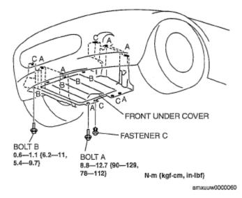
**Fig. 48: Identifying Front Under Cover Components With Torque Specifications Courtesy of MAZDA MOTORS CORP.**
