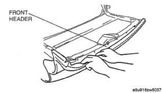
**Fig. 22: Installing Top Fabric To Front Header Courtesy of MAZDA MOTORS CORP.**
