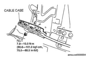
**Fig. 114: Identifying Cable Case And Nut With Torque Specification Courtesy of MAZDA MOTORS CORP.**
