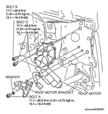
Fig. 70: Identifying Roof Motor Components With Torque Specifications Courtesy of MAZDA MOTORS CORP.
