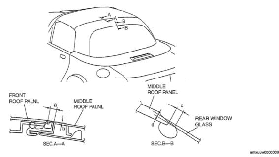
Fig. 59: Identifying Gap And Height Difference Section Between Front Roof Panel And Rear <u>Window Glass</u> Courtesy of MAZDA MOTORS CORP.
