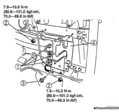
Fig. 115: Removing View Of Power Retractable Hardtop Control Module Bracket With Torque Specifications Courtesy of MAZDA MOTORS CORP.
