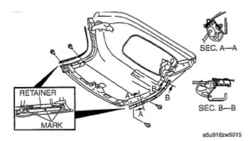
**Fig. 35: Identifying Mark Around Retainer Installation Screws Courtesy of MAZDA MOTORS CORP.**
