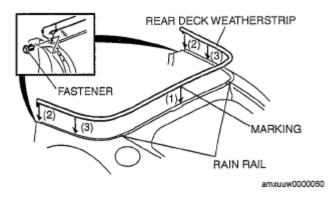
**Fig. 88: Rear Deck Weatherstrip Installation View** Courtesy of MAZDA MOTORS CORP.
