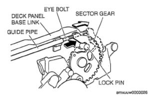
Fig. 129: Disengaging Sector Gear And Lock Pin Of Deck Panel Base Link Courtesy of MAZDA MOTORS CORP.
