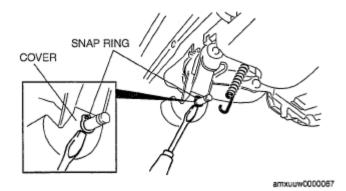
**Fig. 40: Identifying Snap Ring And Cover** Courtesy of MAZDA MOTORS CORP.
