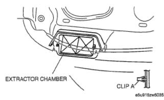
**Fig. 45: Identifying Extractor Chamber And Clip Courtesy of MAZDA MOTORS CORP.**
