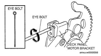
**Fig. 126: Inserting Eye Bolt Into Thread Hole Courtesy of MAZDA MOTORS CORP.**
