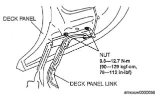
**Fig. 80: Identifying Deck Panel, Deck Panel Link And Nut With Torque Specifications Courtesy of MAZDA MOTORS CORP.**
