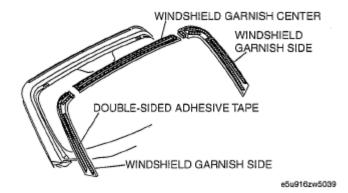
Fig. 30: Identifying Adhesive Tape On Windshield Garnish Courtesy of MAZDA MOTORS CORP.
