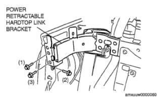
Fig. 102: Power Retractable Hardtop Link Bracket Bolts Tightening Order Courtesy of MAZDA MOTORS CORP.
