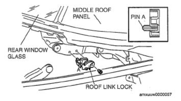
**Fig. 113: Identifying Roof Link Lock Components Courtesy of MAZDA MOTORS CORP.**
