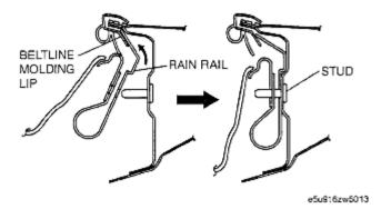
**Fig. 9: Inserting Rain Rail Into Beltline Molding Lip** Courtesy of MAZDA MOTORS CORP.
