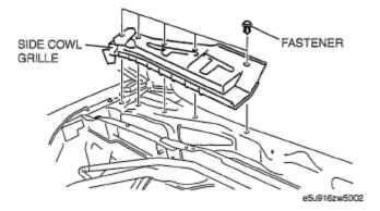
**Fig. 5: Identifying Side Cowl Grille And Fastener Courtesy of MAZDA MOTORS CORP.**
