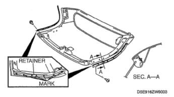
**Fig. 34: Identifying Mark Around Retainer Installation Screws Courtesy of MAZDA MOTORS CORP.**
