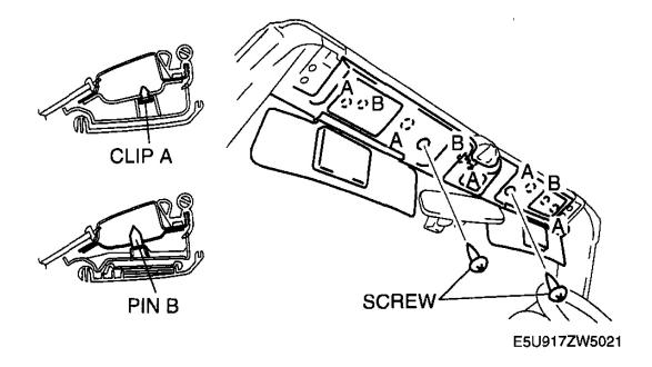
**Fig. 24: Removing Front Header Trim** Courtesy of MAZDA MOTORS CORP.
