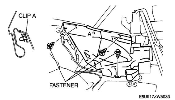
**<u>Fig. 38: Identifying Side Shelf</u>** Courtesy of MAZDA MOTORS CORP.
