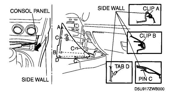
**Fig. 17: Removing Side Wall** Courtesy of MAZDA MOTORS CORP.
