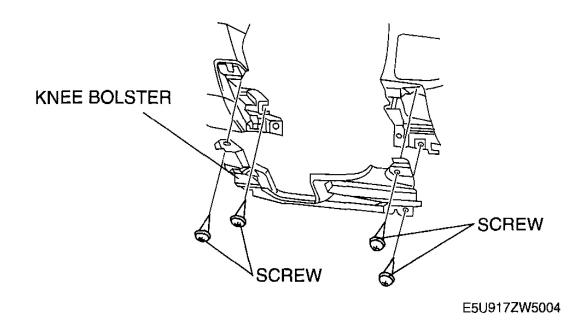
**Fig. 16: Removing Knee Bolster** Courtesy of MAZDA MOTORS CORP.
