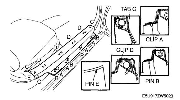
**Fig. 47: Removing Scuff Plate** Courtesy of MAZDA MOTORS CORP.
