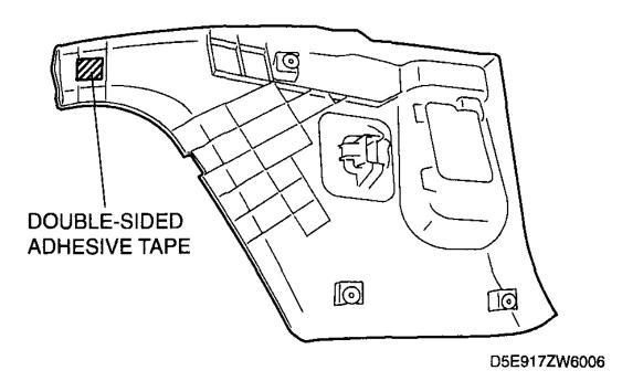
**Fig. 41: Identifying Double-Sided Adhesive Tape To B-Pillar Upper Trim** Courtesy of MAZDA MOTORS CORP.
