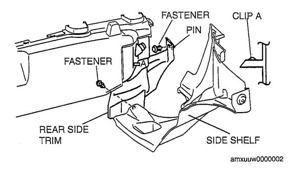
**Fig. 51: Identifying Rear Side Trim & Fasteners** Courtesy of MAZDA MOTORS CORP.
