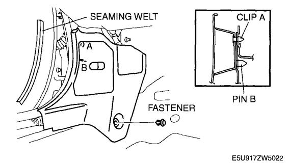
**Fig. 46: Removing Front Side Trim** Courtesy of MAZDA MOTORS CORP.
