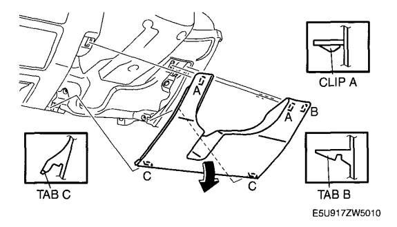
**Fig. 10: Removing Lower Panel** Courtesy of MAZDA MOTORS CORP.
