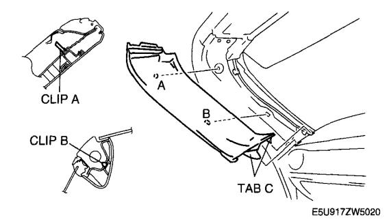
**Fig. 23: Removing A-Pillar Trim** Courtesy of MAZDA MOTORS CORP.
