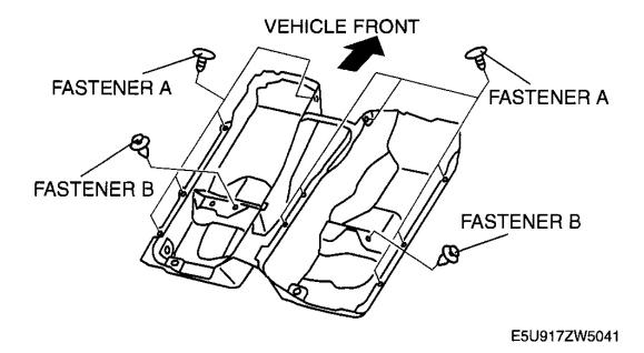
**Fig. 59: Removing Floor Covering Fasteners Courtesy of MAZDA MOTORS CORP.**
