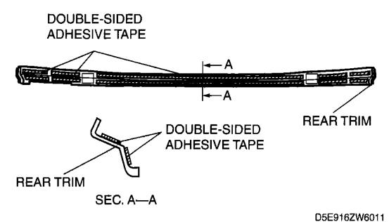
**Fig. 49: Attaching Double-Sided Adhesive Tape To Rear Trim** Courtesy of MAZDA MOTORS CORP.
