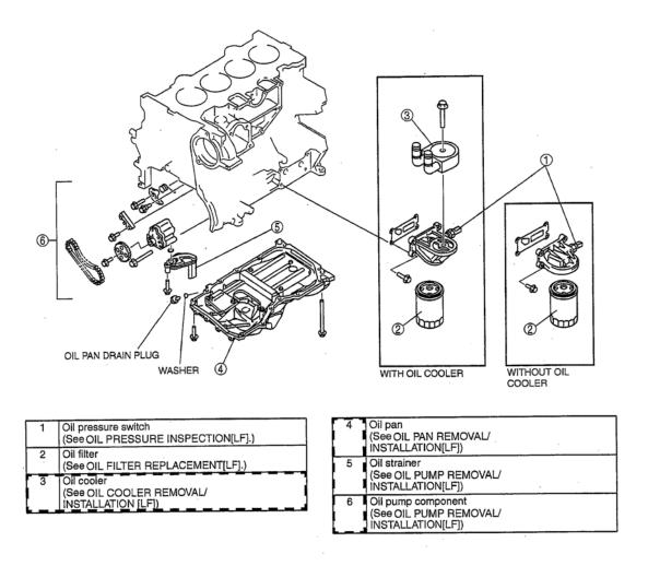
Fig. 1: Identifying Location Of Lubrication System Components Courtesy of MAZDA MOTORS CORP.
