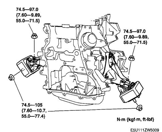
Fig. 8: Identifying Engine Mount Rubber Installation Nuts (With Torque Specifications) Courtesy of MAZDA MOTORS CORP.
