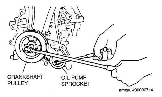
Fig. 16: Installing SST To Oil Pump Sprocket Courtesy of MAZDA MOTORS CORP.
