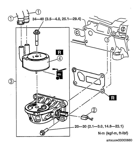
Fig. 18: Identifying Oil Cooler Components Courtesy of MAZDA MOTORS CORP.
