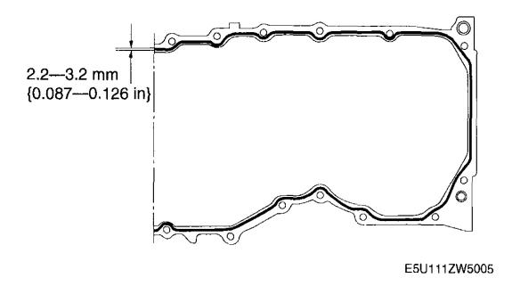
Fig. 12: Applying Silicone Sealant To Oil Pan Courtesy of MAZDA MOTORS CORP.
