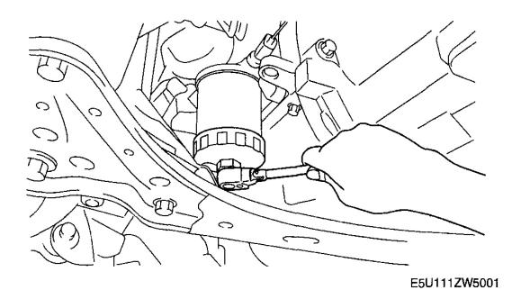
Fig. 5: Removing Oil Filter Courtesy of MAZDA MOTORS CORP.
