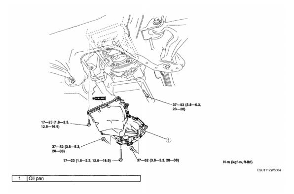
Fig. 6: Identifying Oil Pan Components (With Torque Specifications)
