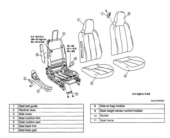
**Fig. 7: Identifying Passenger's Seat Components (With Torque Specifications)** Courtesy of MAZDA MOTORS CORP.
