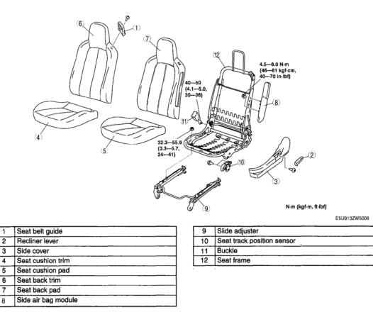
Fig. 6: Identifying Driver's Seat Components (With Torque Specifications) Courtesy of MAZDA MOTORS CORP.
