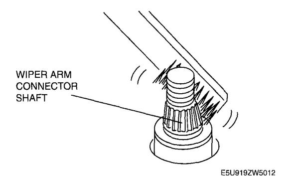
Fig. 3: Cleaning Wiper Arm Connector Shafts Using Wire Brush Courtesy of MAZDA MOTORS CORP.
