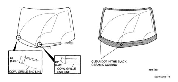
Fig. 4: Identifying Wiper Arm & Blade Slide Area Courtesy of MAZDA MOTORS CORP.
