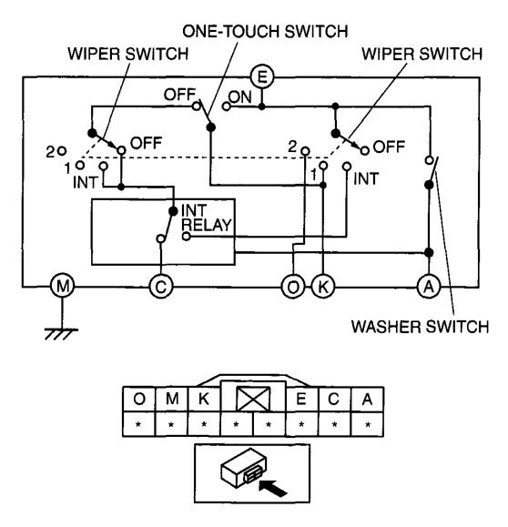
Fig. 18: Identifying Wiper & Washer Switch Circuit Courtesy of MAZDA MOTORS CORP.
