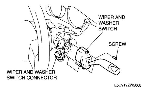
Fig. 16: Removing Wiper & Washer Switch Courtesy of MAZDA MOTORS CORP.
