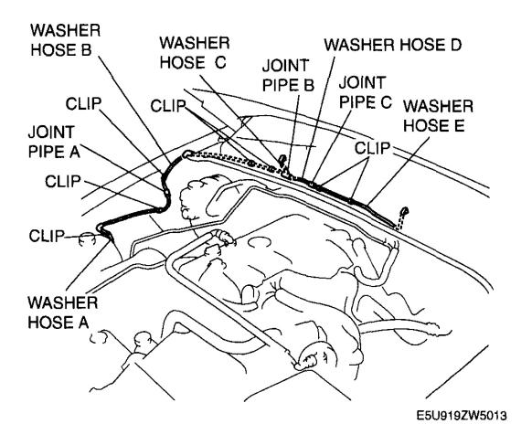
Fig. 15: Removing/Installing Washer Hose Courtesy of MAZDA MOTORS CORP.
