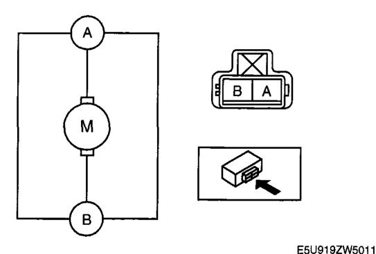
Fig. 13: Identifying Washer Motor Connector Courtesy of MAZDA MOTORS CORP.
