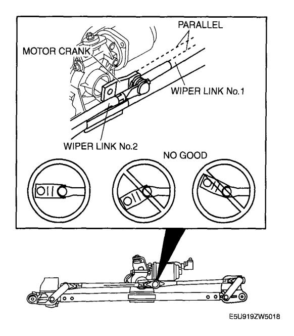
Fig. 8: Identifying Propper Wiper Link Adjustment Courtesy of MAZDA MOTORS CORP.
