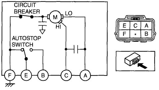
Fig. 9: Identifying Wiper Motor Circuit Courtesy of MAZDA MOTORS CORP.
