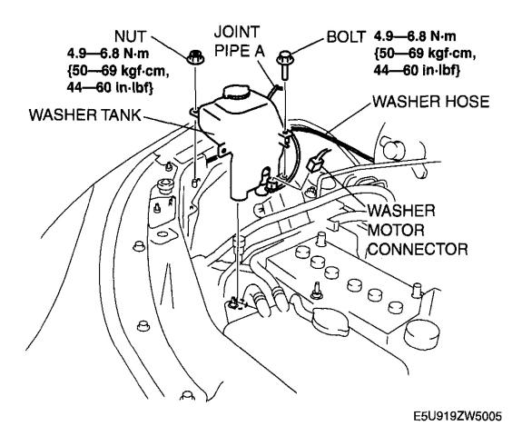
Fig. 11: Washer Tank (With Torque Specifications) Courtesy of MAZDA MOTORS CORP.
