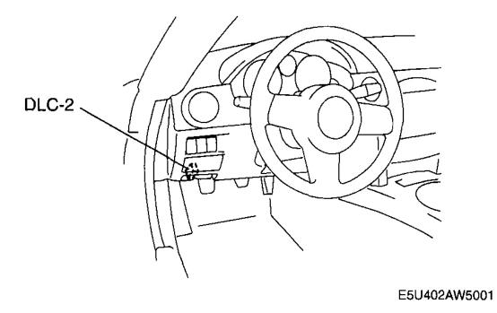
Fig. 13: Locating DLC-2 Connector Courtesy of MAZDA MOTORS CORP.
