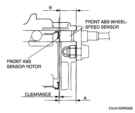
Fig. 12: Measuring Distance Between Front ABS Wheel-Speed Sensor Installation Surface & ABS Wheel-Speed Sensor Tip
