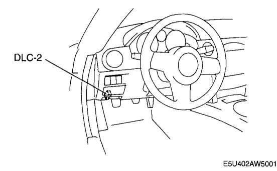
Fig. 3: Locating DLC-2 Connector Courtesy of MAZDA MOTORS CORP.
