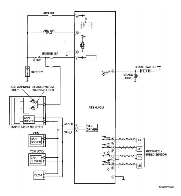
Fig. 2: ABS System Wiring Diagram Courtesy of MAZDA MOTORS CORP.
