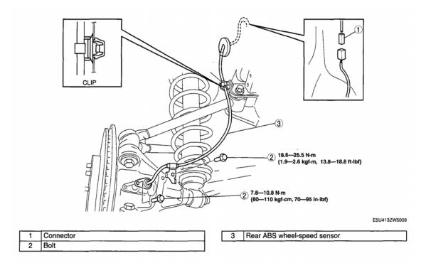
Fig. 14: Identifying Rear ABS Wheel-Speed Sensor (With Torque Specifications) Courtesy of MAZDA MOTORS CORP.
