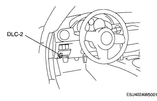
Fig. 9: Locating DLC-2 Connector Courtesy of MAZDA MOTORS CORP.
