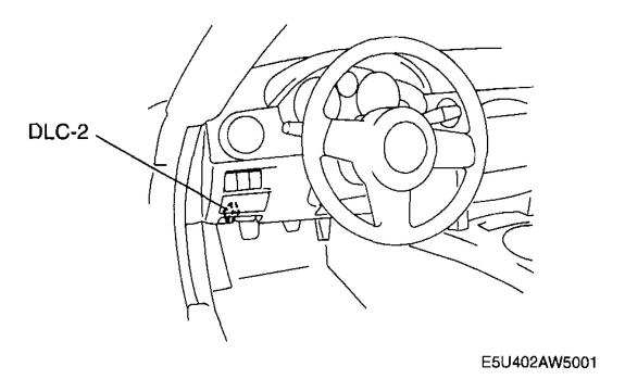
Fig. 16: Locating DLC-2 Connector Courtesy of MAZDA MOTORS CORP.
