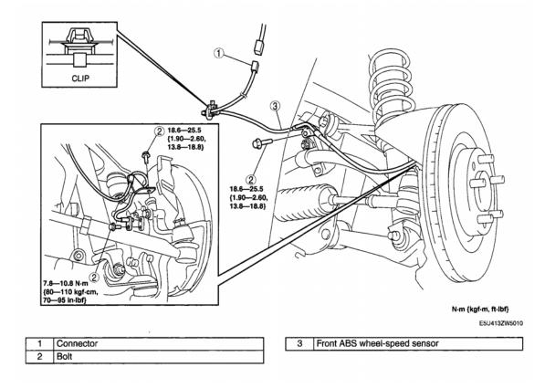
Fig. 11: Identifying Front ABS Wheel-Speed Sensor (With Torque Specifications) Courtesy of MAZDA MOTORS CORP.
