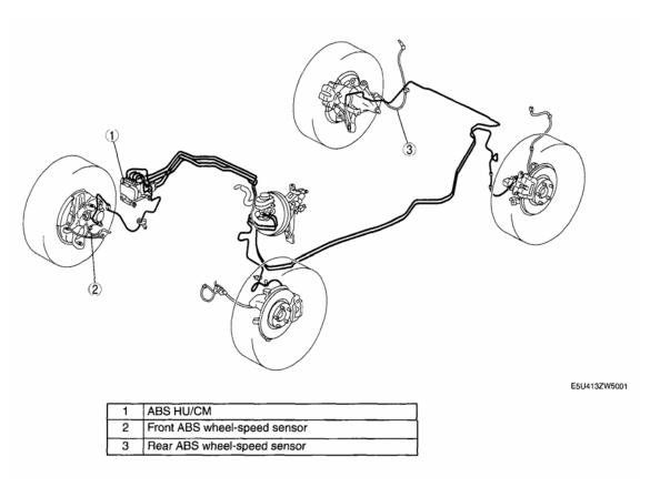
Fig. 1: Identifying Location Of ABS Components Courtesy of MAZDA MOTORS CORP.
