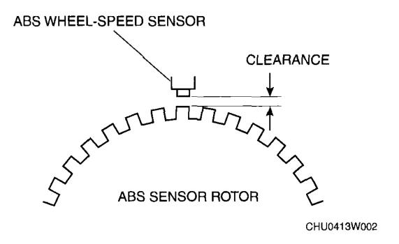
Fig. 15: Inspecting ABS Sensor-To-Rotor Clearance Courtesy of MAZDA MOTORS CORP.
