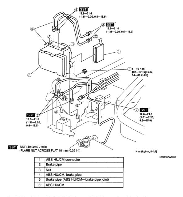
Fig. 4: Identifying ABS HU/CM Steps (With Torque Specifications) Courtesy of MAZDA MOTORS CORP.
