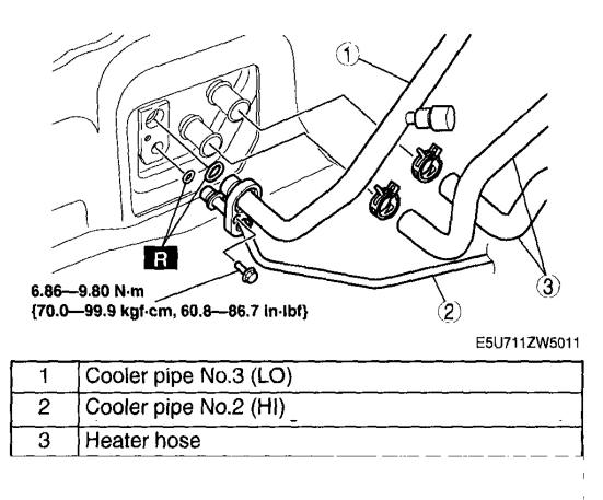
Fig. 6: View Of Refrigerant Line From A/C Unit & Components (With Torque Specifications) Courtesy of MAZDA MOTORS CORP.
