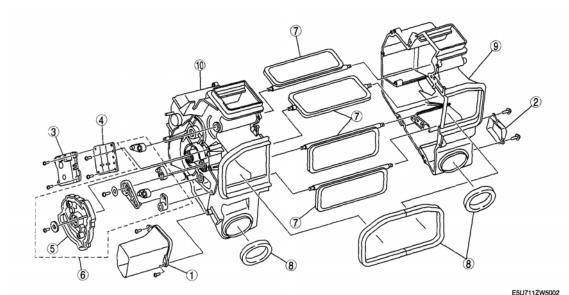
Airflow mode link set 6 Duct (1) 7 Airflow mode door Duct (2) 2 8 Polyurethane form Airflow mode actuator з Case (1) 9 4 Bracket Airflow mode main link 10 Case (2) 5
