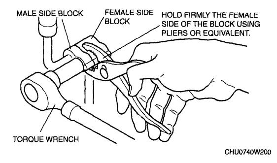
**Fig. 15: Disconnecting Block Joint Type Pipes Courtesy of MAZDA MOTORS CORP.**
