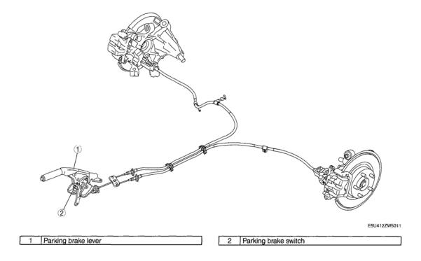
Fig. 1: Identifying Parking Brake System Components Courtesy of MAZDA MOTORS CORP.
