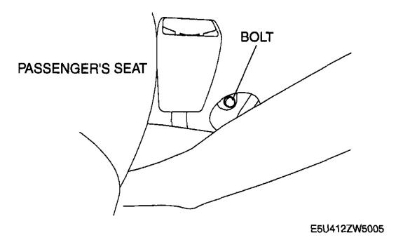
Fig. 5: Locating Bolt Courtesy of MAZDA MOTORS CORP.
