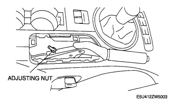
Fig. 3: Identifying Parking Brake Lever Adjusting Nut Courtesy of MAZDA MOTORS CORP.
