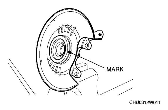
Fig. 11: Placing Alignment Mark On Dust Cover & Rear Knuckle Courtesy of MAZDA MOTORS CORP.
