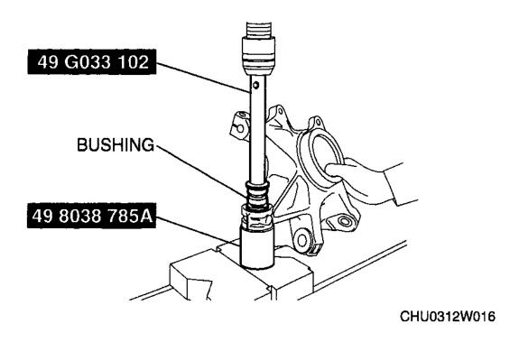
Fig. 16: Pressing New Bushing Into Rear Knuckle Using SST's Courtesy of MAZDA MOTORS CORP.
