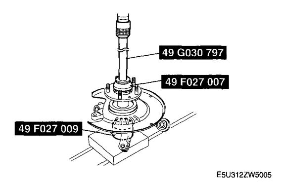
Fig. 20: Installing Wheel Hub Components Using SST's Courtesy of MAZDA MOTORS CORP.
