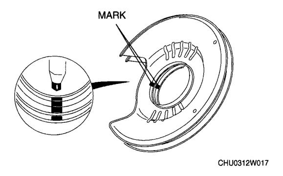
Fig. 17: Aligning Marks On New Dust Cover & Rear Knuckle Courtesy of MAZDA MOTORS CORP.
