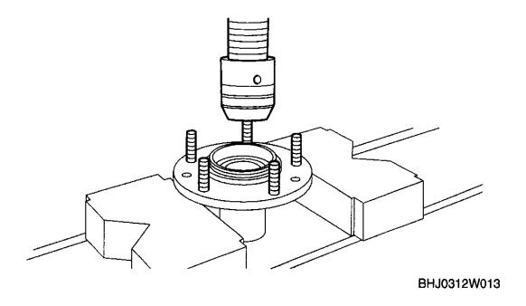
Fig. 14: Removing Wheel Hub Bolts From Wheel Hub Using Press Courtesy of MAZDA MOTORS CORP.
