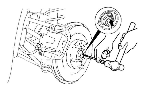
Fig. 4: Knocking Out Crimped Portion Of Locknut Outward Using Chisel & Hammer Courtesy of MAZDA MOTORS CORP.
