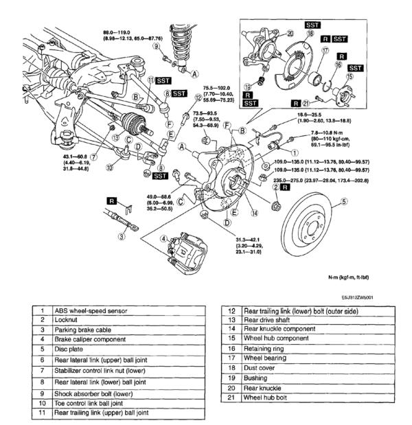
Fig. 3: Identifying Wheel Hub Components (With Torque Specifications) Courtesy of MAZDA MOTORS CORP.
