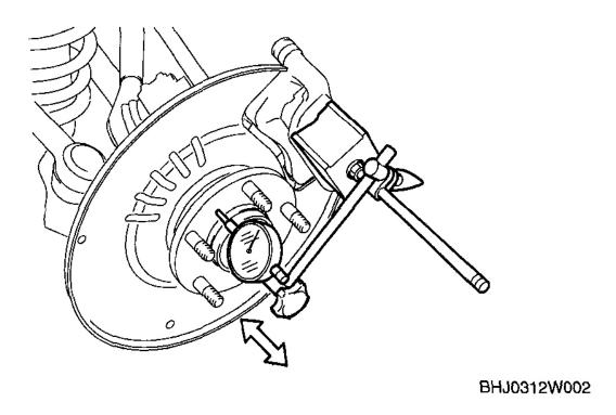
Fig. 2: View Of Magnetic Vase & Dial Gauge Courtesy of MAZDA MOTORS CORP.
