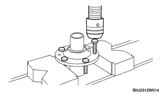
Fig. 15: Pressing New Wheel Hub Bolts Into Wheel Hub Using Press Courtesy of MAZDA MOTORS CORP.
