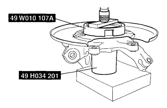
Fig. 18: Pressing New Dust Cover Onto Rear Knuckle Using SST's Courtesy of MAZDA MOTORS CORP.
