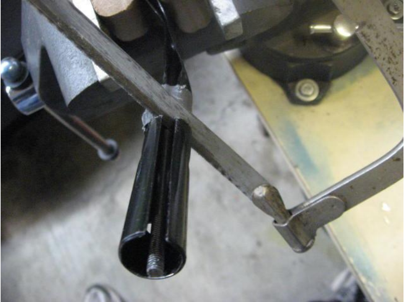
Figure 15 – Cut the lever tube and release rod with a hacksaw
