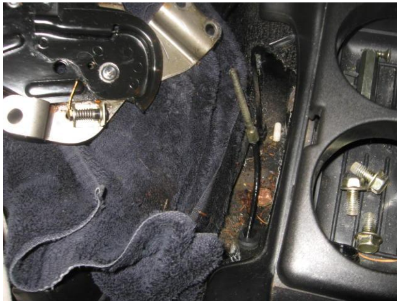
Figure 11 – Remove brake cable and pull lever assembly from vehicle
