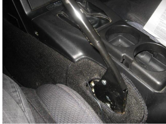
Figure 5 – Lever with handle removed
