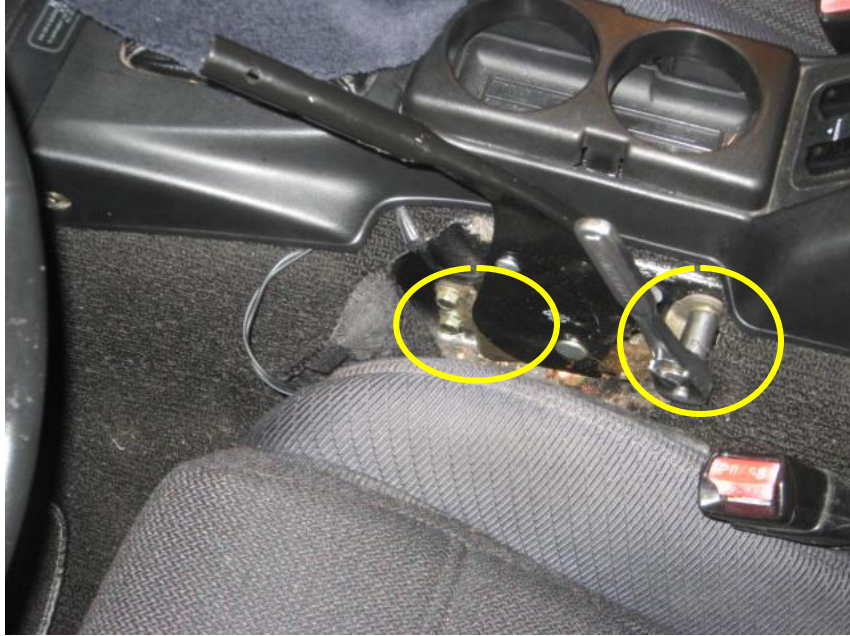
Figure 8 – Parking lever assembly bolts (that's a socket wrench on the single bolt)
