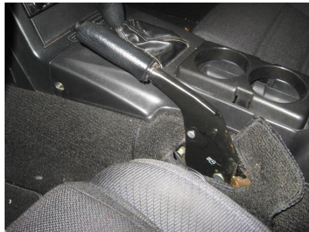
Figure 3 – Lever with cover assembly removed
