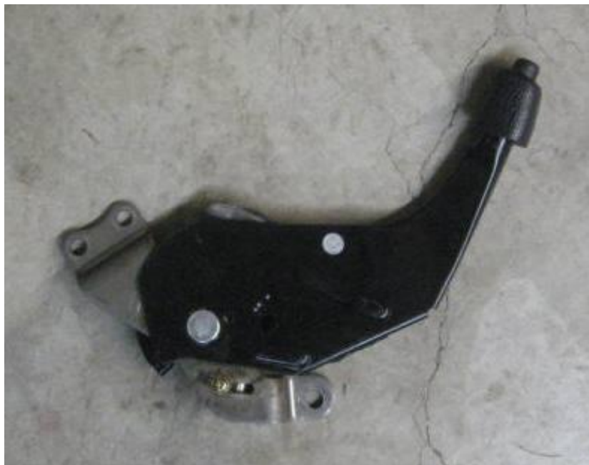
Figure 22 – Reassembled brake lever assembly.
