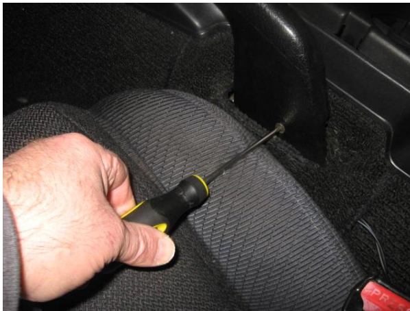
Figure 2 – Remove screw to separate cover halves
