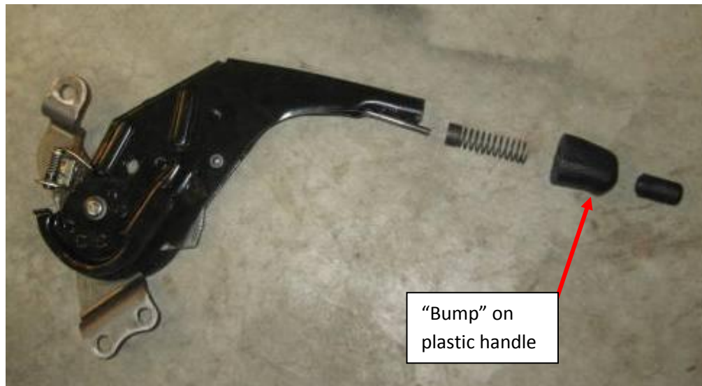
Figure 21 – Proper orientation of parts for reassembly
