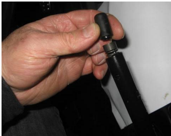
Figure 6 – Remove the release button and spring
