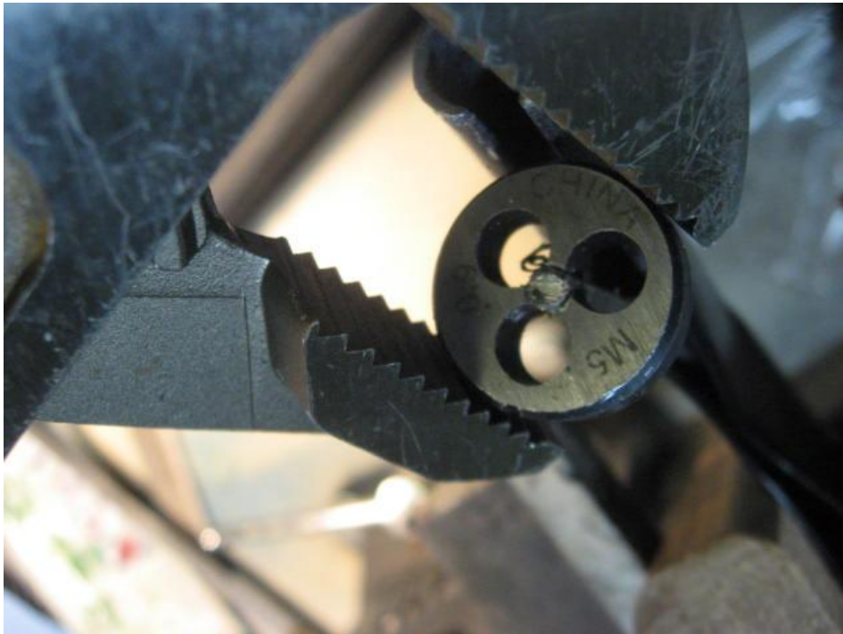
Figure 16 – Cut new threads with an M5 die and channel locks
