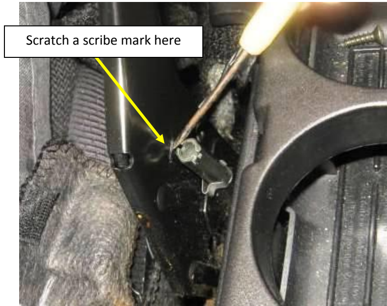
Figure 10 – Adjustment screw scribe mark
