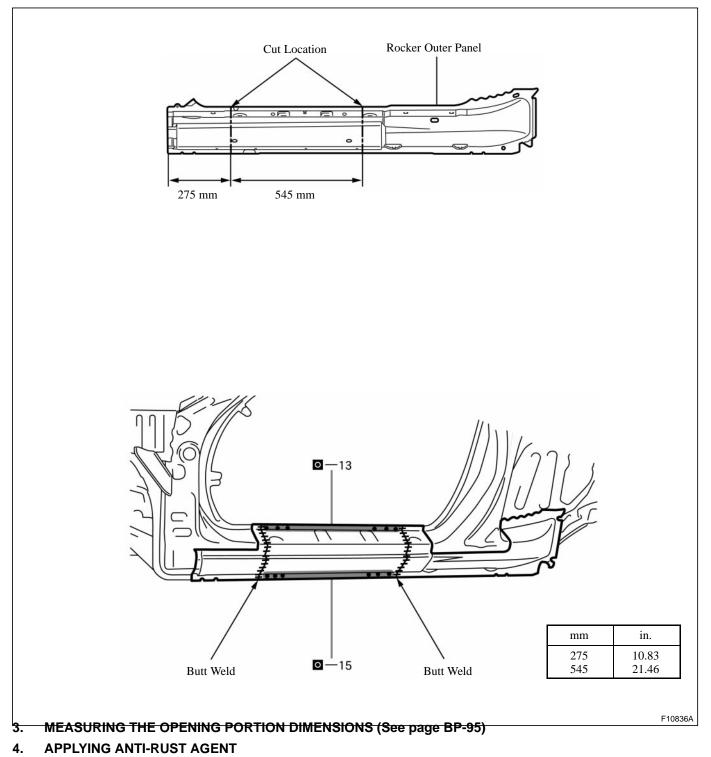
(a) After applying the top coat layer, apply the anti-rust agent to the inside of the necked section structural weld spots.
