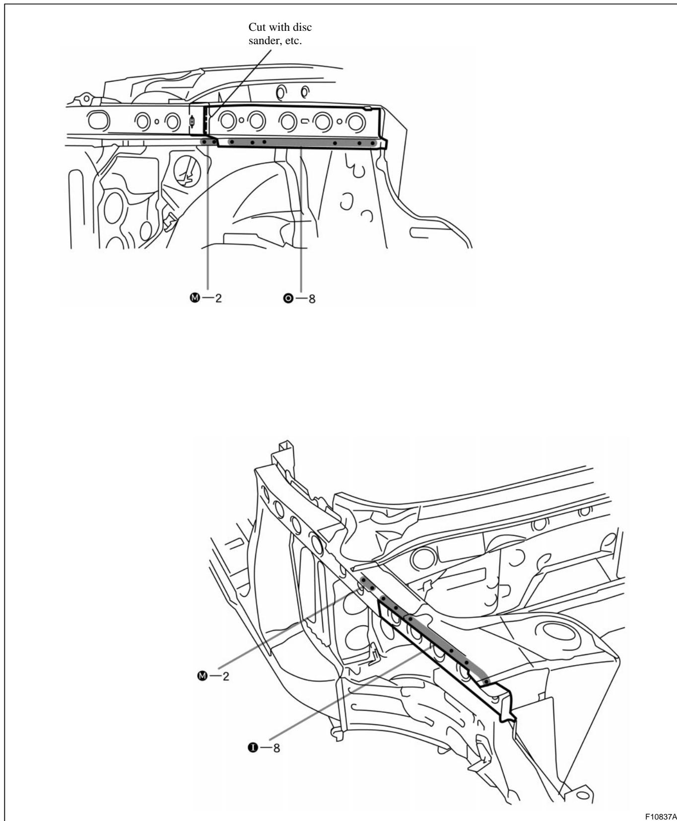
3. INSTALL SIDE PANEL NO.4 REINFORCEMENT
