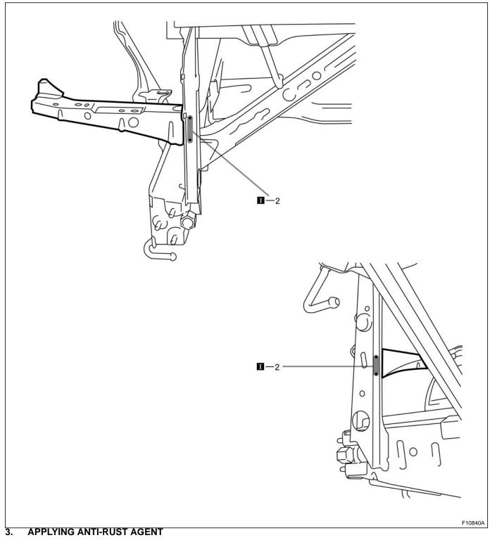
(a) After applying the top coat layer, apply the anti-rust agent to the inside of the necked section structural weld spots.
