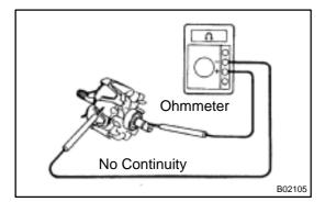
(b) Check the rotor for ground.Using an ohmmeter, check that there is no continuity between the slip ring and rotor.
