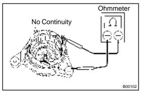
(b) Check the stator for ground.Using an ohmmeter, check that there is no continuity between the coil lead and drive end frame.
