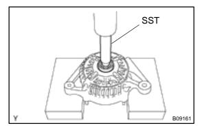
(b) Using SST and a press, press out the bearing. SST 09950–60010 (09951–00350), 09950–70010 (09951–07100)
