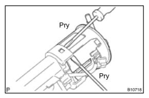
(b) Using 2 screwdrivers, pry out the fuel suction plate.
