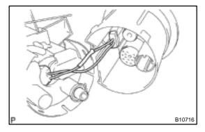
(c) Disconnect the fuel pump connector.
