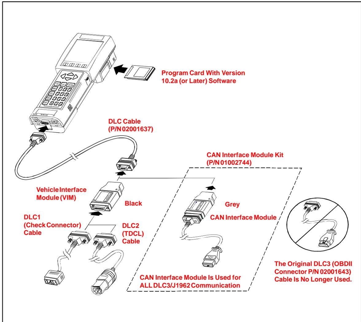
1. Remove the original DLC3 Cable and store it in the Diagnostic Tester storage case.
