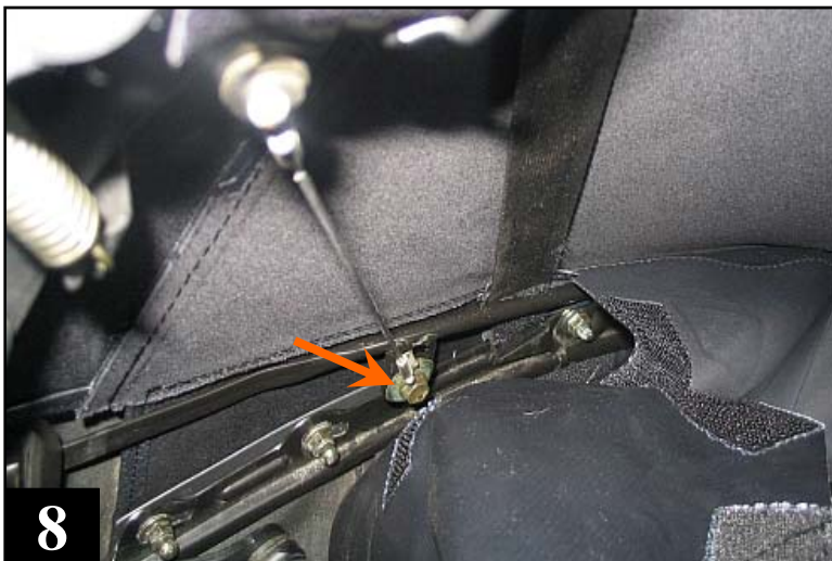
8 Connect rear bow locator cable to rear qtr. brackets. Tighten nuts onto all sections across rear assy.
