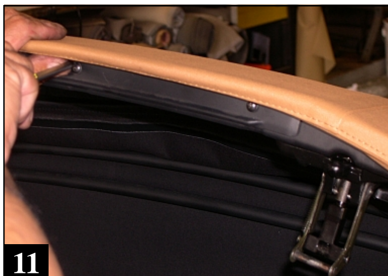
11 Install retainer across header bow (6 philips screws)
