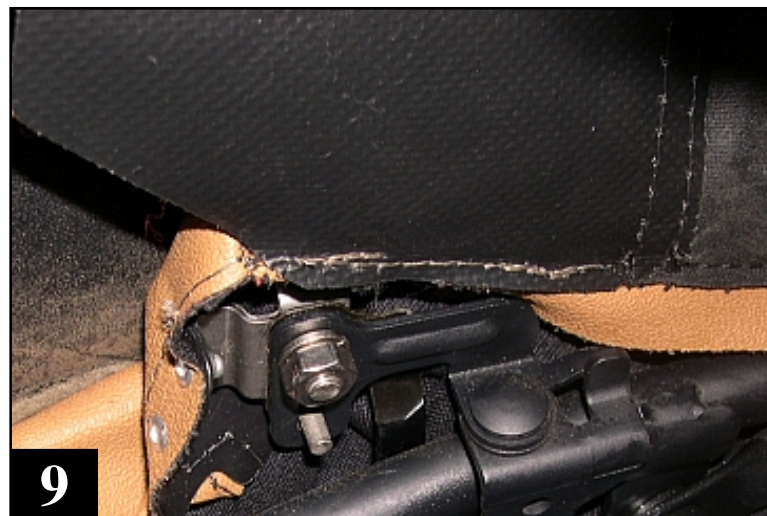
9 Attach side tension cable end brackets to L&R quarters.
