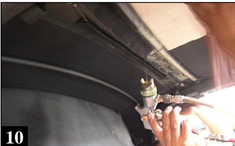
10 Apply adhesive to # 2 bow. Slip sleeve w/velcro over spring on cable. Adhere flap of material along front edge of sleeve to #2 bow.
