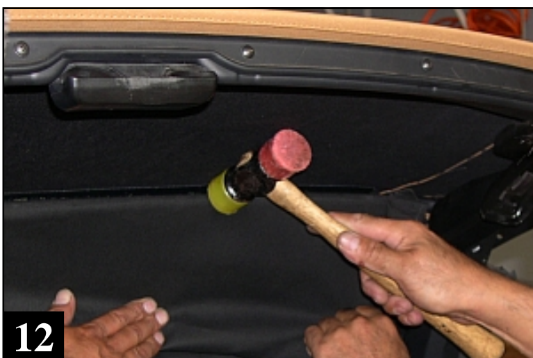
12 Insert plastic edge of large listing panel into channel on #2 bow and tap channel closed to secure.
