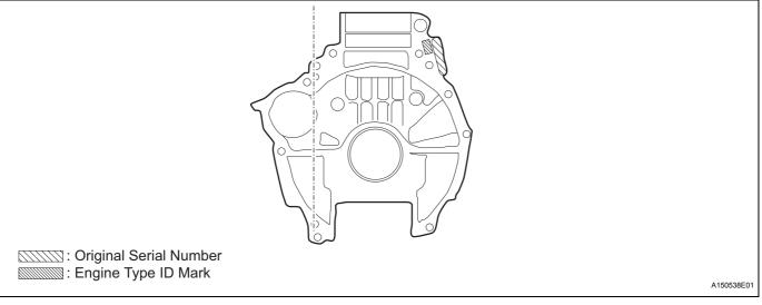
A new serial number has been engraved by needle marker into the lower crankcase as shown on the drawing.
