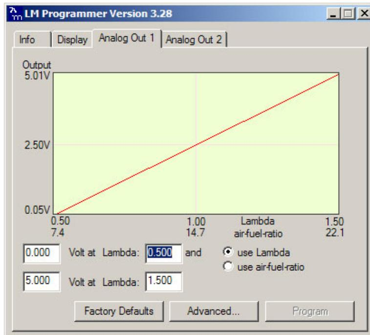
This shows the analog output voltages versus Lambda for one of the two analog outputs. The graph display is automatically scaled to the selected voltages. For each output you can specify a minimum and maximum lambda or A/F ratio value and the associated voltages. Below the minimum and above the maximum values the output voltages stay constant at the associated programmed voltage.
