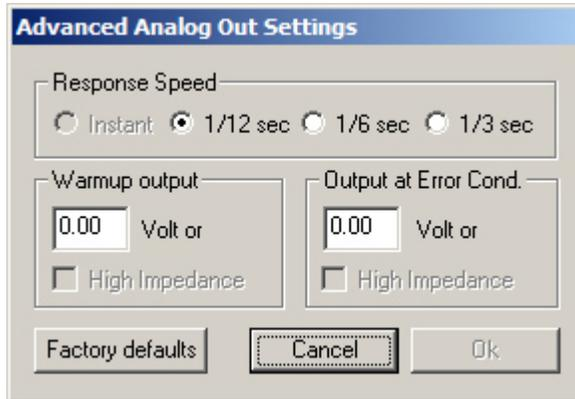
When setting the MTX-L to the slower response speed settings the measured mixture data will be averaged over the response time setting before being sent via the analog output.
